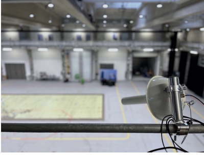
Figure 15: GNSS repeater in the Fraunhofer test-center.
