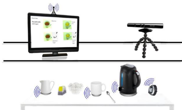
Figure 1: Schematic illustration of the CogWatch Prototype 1.2 System showing VTE display (top left), Kinect Motion system (top right), wrist-watch device (bottom right), instrumented tea-making items (bottom left and middle).
