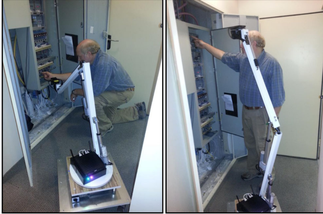
Figure 7. TeleAdvisor’s second prototype robotic arm has a wide range reach.
