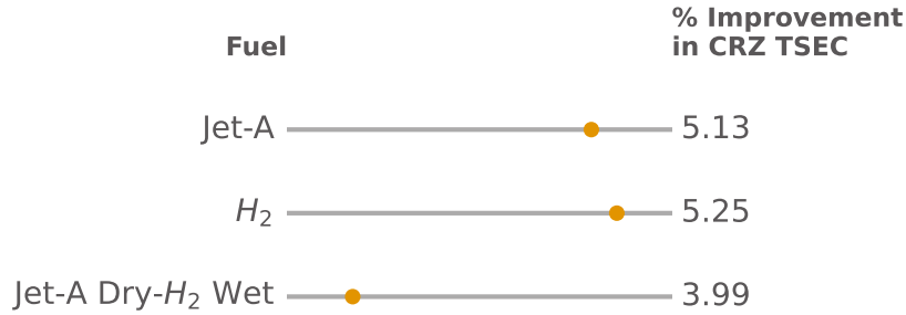
Fig. 9 Percent relative improvement in thrust specific energy consumption (TSEC) of the N+3 engine with water recovery. This plot compares the relative improvement of the two optimization problems with water recovery compared to the optimization problems without water recovery. The relative performance of hydrogen with water recovery compared to Jet-A without water recovery is also shown.
