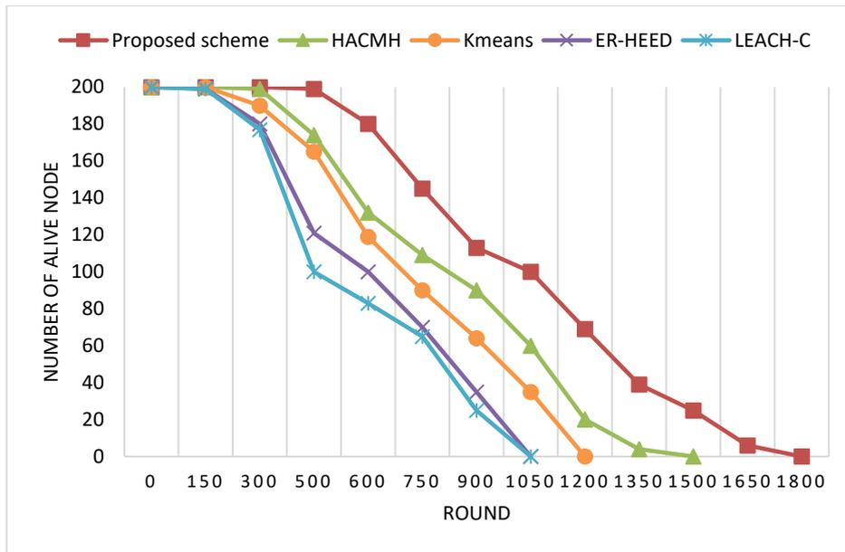
Fig. 3. Distribution of alive sensor nodes according to the number of rounds for each algorithm
