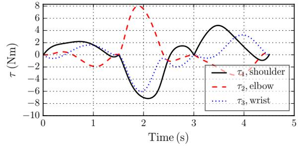
Fig. 4. The right arm torque profiles for case 1.
