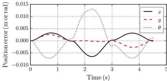
Fig. 8. Position tracking errors when time-delayed estimation is used for the dynamics parameters of the object.
