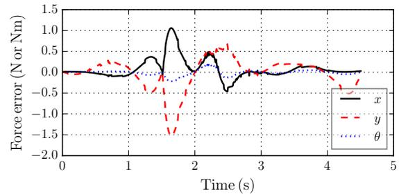
Fig. 9. Constraint force prediction errors when time-delayed estimation is used for the dynamics parameters of the object.
