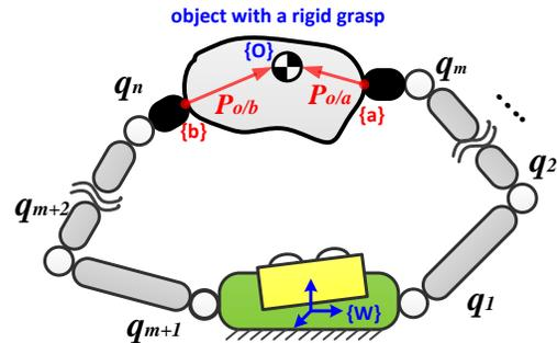
Fig. 1. A schematic diagram of the bimanual manipulation of a common object, where the detailed symbol representations are indicated in Section II.
