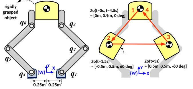
Fig. 2. Planar bimanual object manipulation system, and the reference task properties.
