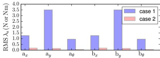
Fig. 7. RMS values of the internal (squeeze) constraint force when minimizing a quadratic cost in control command (case 1) and constraint force (case 2).
