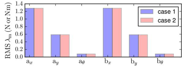
Fig. 6. RMS values of the motion-inducing constraint force when minimizing a quadratic cost in control command (case 1) and constraint force (case 2).
