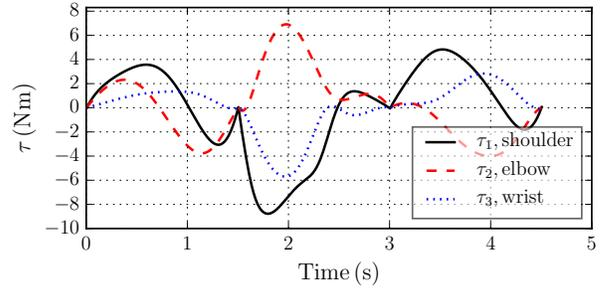
Fig. 5. The right arm torque profiles for case 2.
