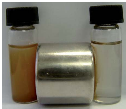
Fig. 6 Photograph of the samples in a magnetic field. On the left is the iron hydroxide nanostructures and on the right is the iron oxide nanostructures.
