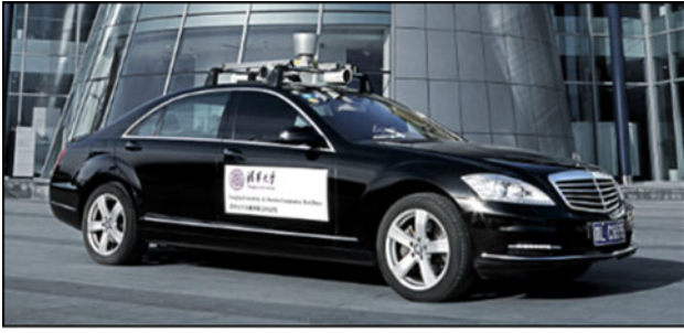
Fig. 7. Vehicle platform (the vehicle platform includes a 360° laser LIDAR, four external cameras, one internal camera, the CAN information, and data storing computer).
