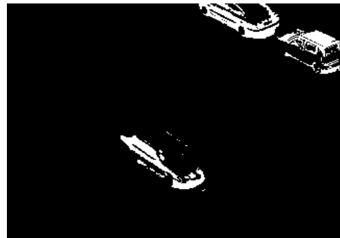
(b) Motion detection by simple back ground subtraction
