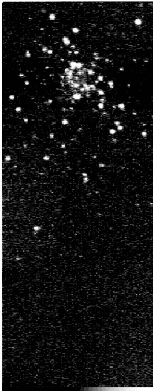
FIG. 59. IR FOV during scan of 47 Tuc. The FOV is 100 scans wide and 512 physical pixels tall. To have matching spatial scale in both directions, the image has been stretched by a factor of 2 in the scan (horizontal) direction.
