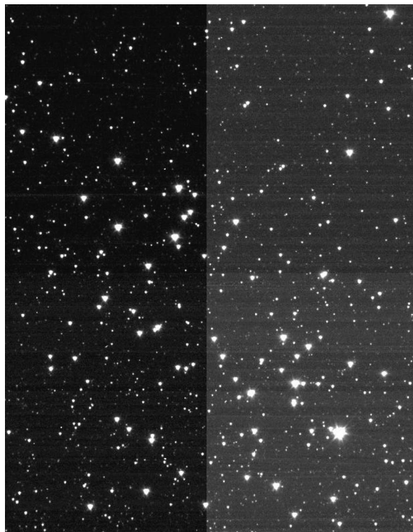
FIG. 14. Central strip of the MRI alignment image of star cluster NGC 3532, taken 2 days after launch, heavily stretched to show dimmest star images, noise, and bias differences in the four quadrants. Note the triangular shape of the heavily overexposed images due to stressing of the optics by the mounts and six offset diffraction spikes due to the nonradial secondary mount spider vanes.
