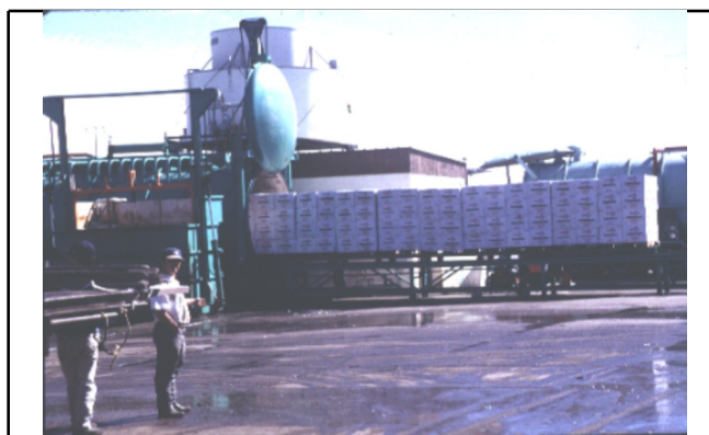
Fig. 6. Large shippers can cool a wide range of vegetables using vacuum cooling.
