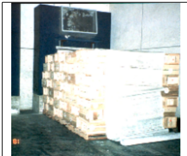
Fig. 4. Portable forced-air coolers can be operated in the field.
