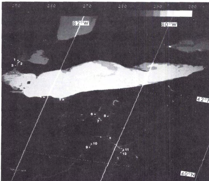
FIG. 1. NOAA-6 3.8- \mu\text{m} image of the midwestern United States taken on 24 September 1979 at 0015 GMT. The high temperature areas appear white and are identified in Table 2. Imagery processed by NASA/GSFC, Code 942.
