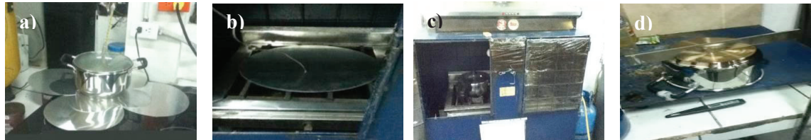
Fig. 1 a) Image of the discs used for the energy efficiency with different heights test. b) Image of aluminium disk over a heat source. c) Image of the pot under thermal impact conditions. d) Image of the concavity measurement process.
