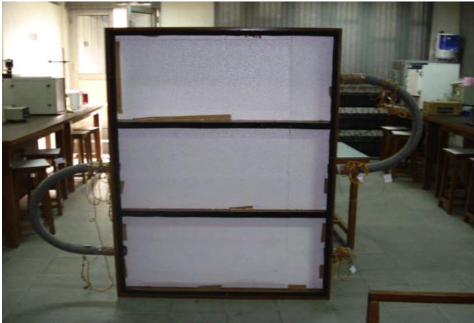
Fig. 9: Photograph of Wooden Duct with Air Flow Configuration [6].
