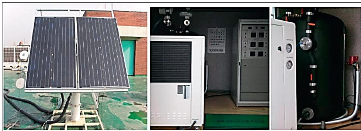
Fig. 17: Experimental View of the PV/T System and the PV Module; Measuring Equipment [10].
