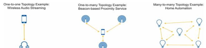
Fig. 4. Three examples of three kinds of topologies of Bluetooth [9]
