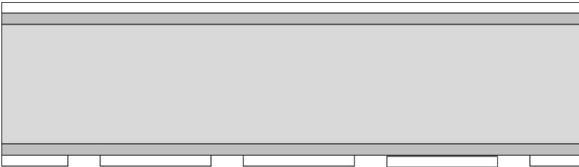
Figure 3.3.3. Cross section of an n-type silicon wafer during J_{0,met} test structure processing, after contact opening lithography (not to scale).
