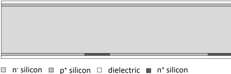
Figure 1.4.2.2. Schematic representation of the state of a device wafer during IBC solar cell processing, after BSF oxidation.
