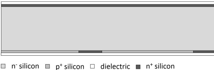
Figure 1.4.2.3. Schematic representation of the state of a device wafer during IBC solar cell processing, after FSF oxidation.
