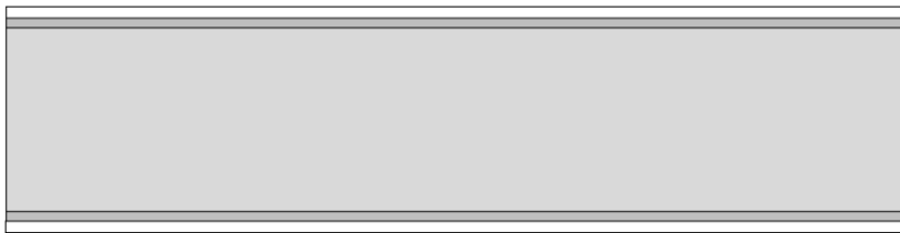
Figure 1.4.2.1. Schematic representation of the state of a device wafer during IBC solar cell processing, after emitter oxidation.
