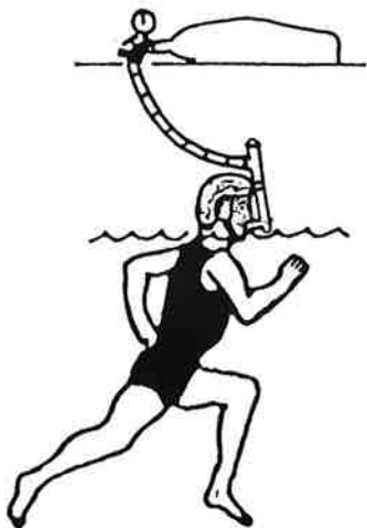
Figure 1—Schematic drawing of the expired air collection procedure during supported running in water.
