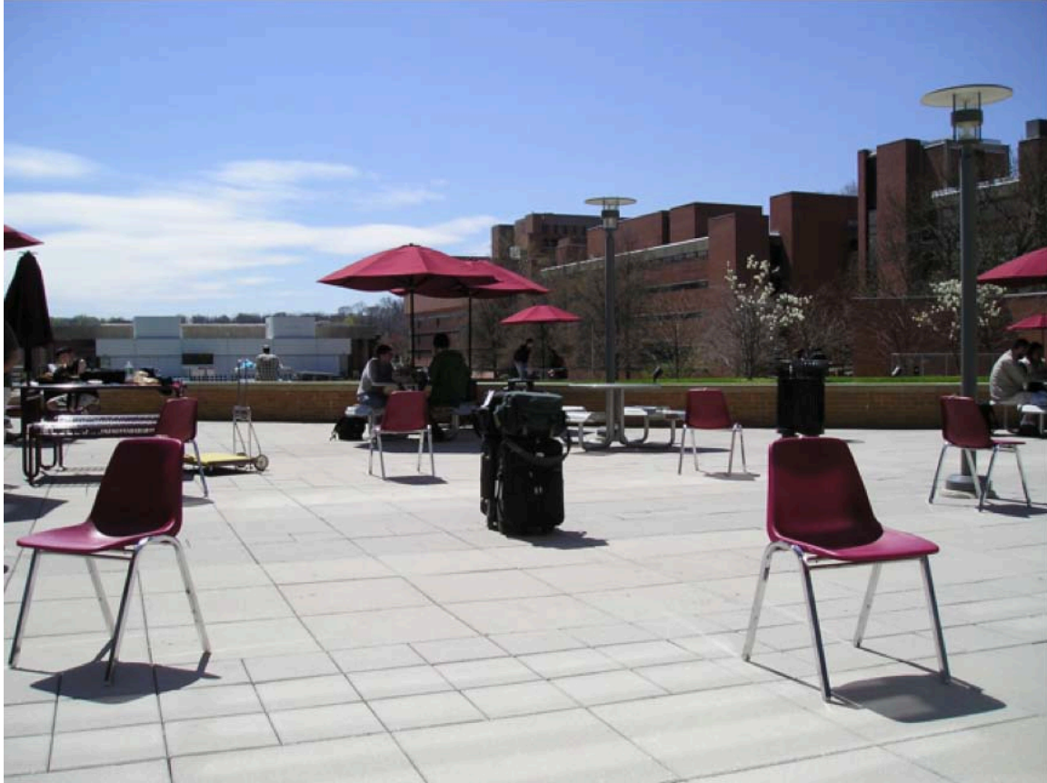
Figure 1. Smoldering cigarettes arrayed on 8 chairs in a ring about the air quality monitors in luggage bags at the center, such that no matter which way the wind blows in any of 8 compass directions, the smoke from one cigarette will be detected by the monitors (Repace, 2005). Atmospheric conditions were turbulent, with strong sun and high wind speeds, ranging from 5 m/s to 10 m/s (11 MPH to 23 MPH).
