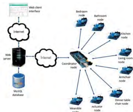
Figure 1: Architecture of the considered environmental sensor network (picture taken from (Dasios et al., 2015)).
