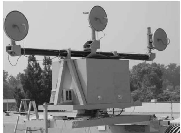
Figure 5. Photograph of the interferometric radar used for long-range AOA measurements.
