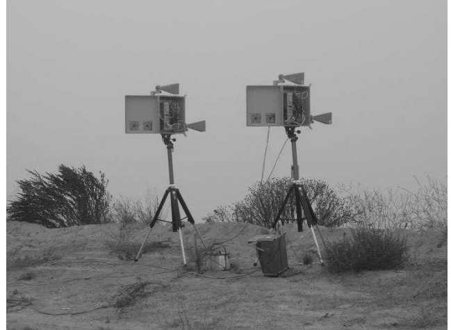
Figure 4. Photograph of the repeaters used for short-range AOA and C_n^2 measurements.
