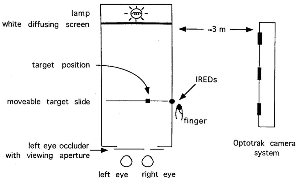
Figure 1. A schematic representation of the experimental apparatus.
