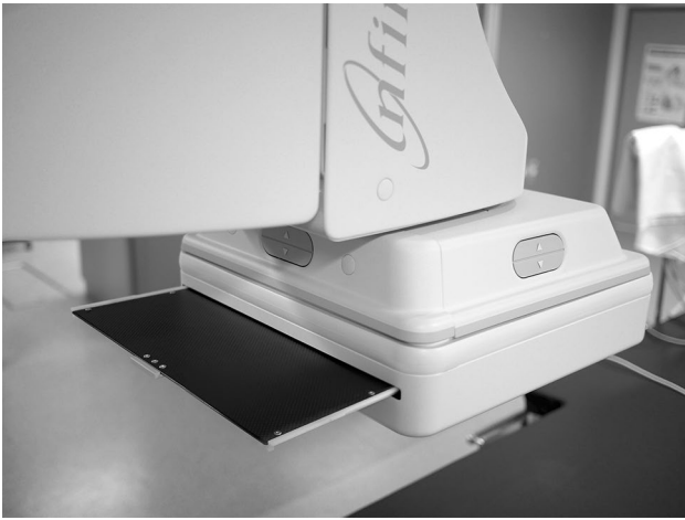
Fig. 1 The anti-scatter grid (ASG) can be removed or re-inserted rapidly from the input of the imaging detector
