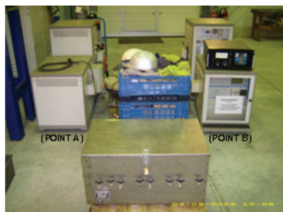
Figure 20: Layout of analysis system RWTH (left), RWTH off-gas measurement equipment (point A and point B) (right)
