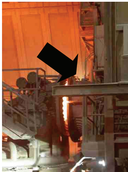
Figure 19: Location of the sampling probes at point A (composition and temperature) in the movable elbow near the EAF
