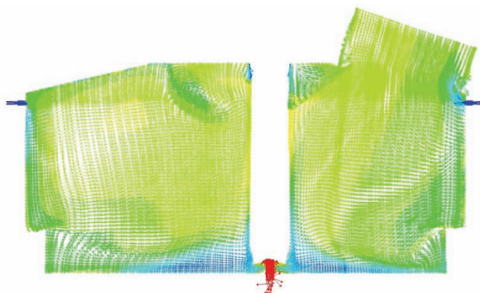
a) Vector Plot: Temperature distribution in cross-section through centre of off-gas duct
