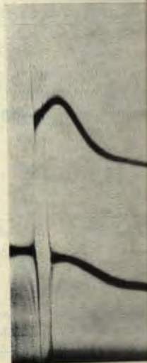
Fig. 5. Ultracentrifugation pattern of lysate. Two peaks were noted, as demonstrated in this pattern. The sedimentation coefficient of the slower peak was 1.75. The upper peak contained material remaining after a 100,000 rpm centrifugation.
