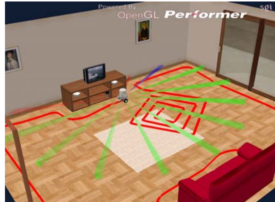
Figure 9: Virtual Prototype: a) General view with a random object; b) Swept area.
