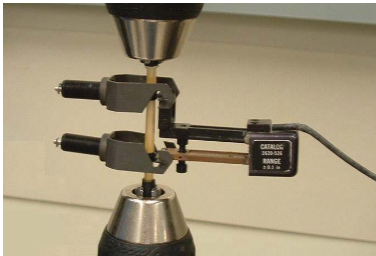
Figure 2. Tension test setup for wheat/barley specimens. The picture shows the load frame jaws, the end grips, the heat shrink collars, and the extensometer.
