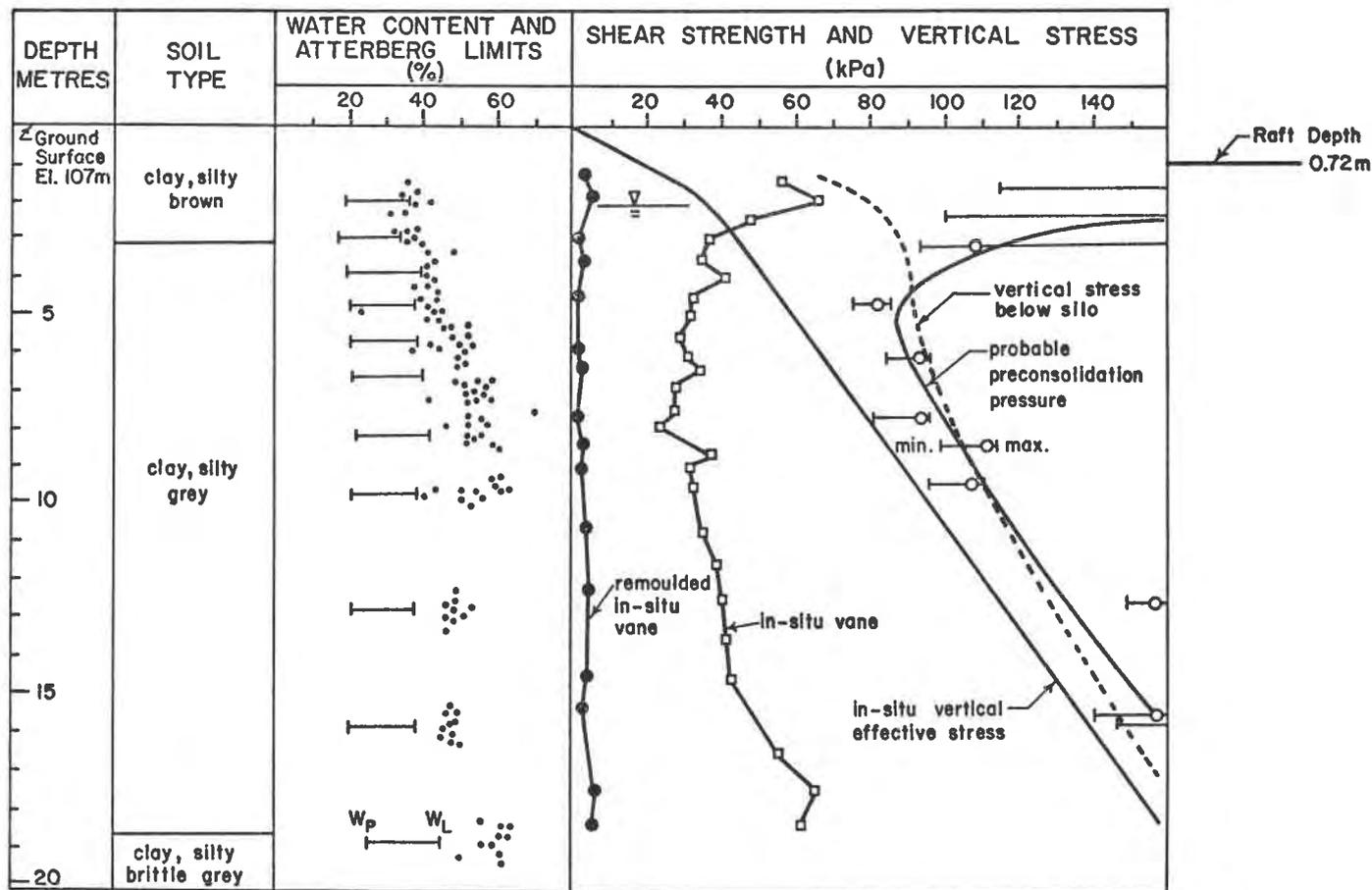
Figure 1. Soil profile at raft location.
