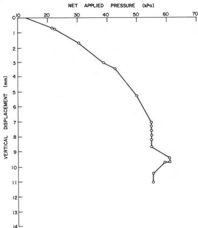
Figure 4. Settlement of silo raft foundation.
