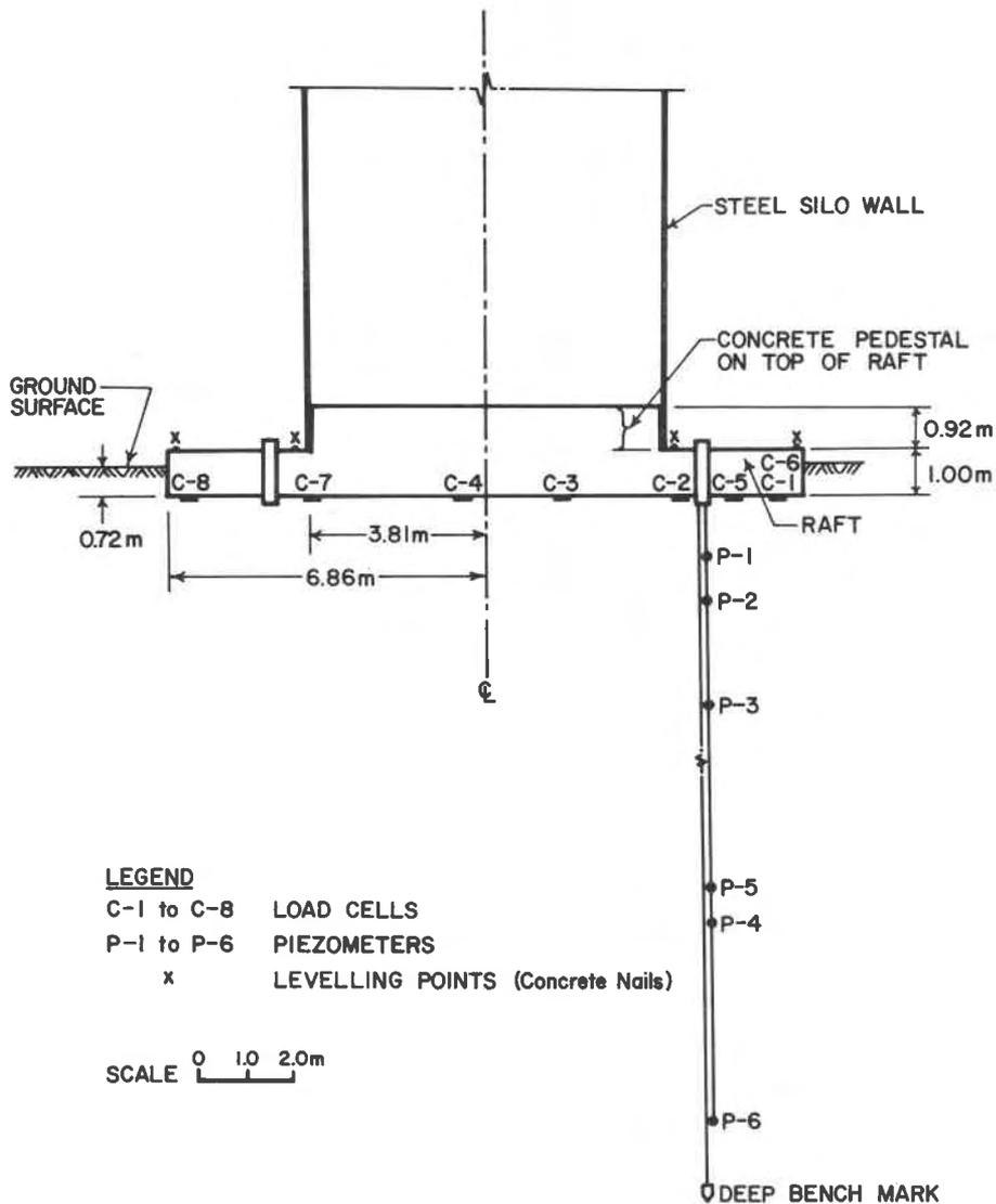
Figure 3. Section through silo, showing foundation and instrumentation.
