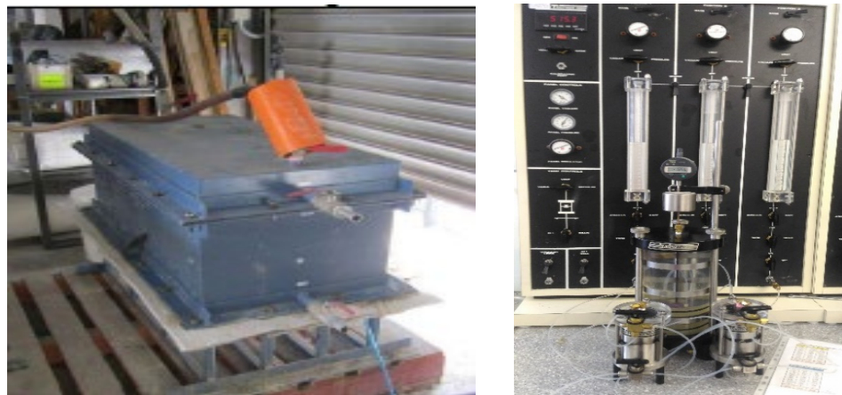
Figure 4 – Laboratory test setups; (i) Model scale Flow box setup (ii) Element scale Permeameter cell setup
