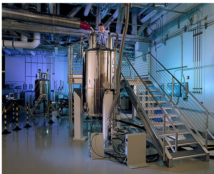
Pacific Northwest National Laboratory's high magnetic field (800 MHz) NMR spectrometer being loaded with a sample.
