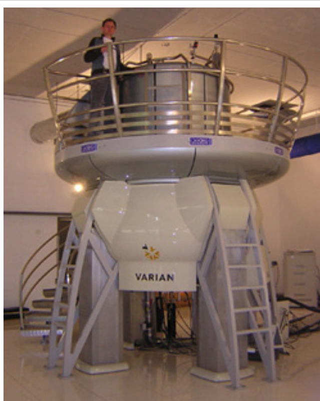
A 900MHz NMR instrument with a 21.2 T magnet at HWB-NMR, Birmingham, UK
