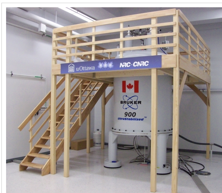
Solid-state 900 MHz (21.1 T [1] ) NMR spectrometer at the Canadian National Ultrahigh-field NMR Facility for Solids.
