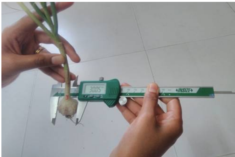
Fig. 4. Measurement of Equilateral Diameter of Garlic
