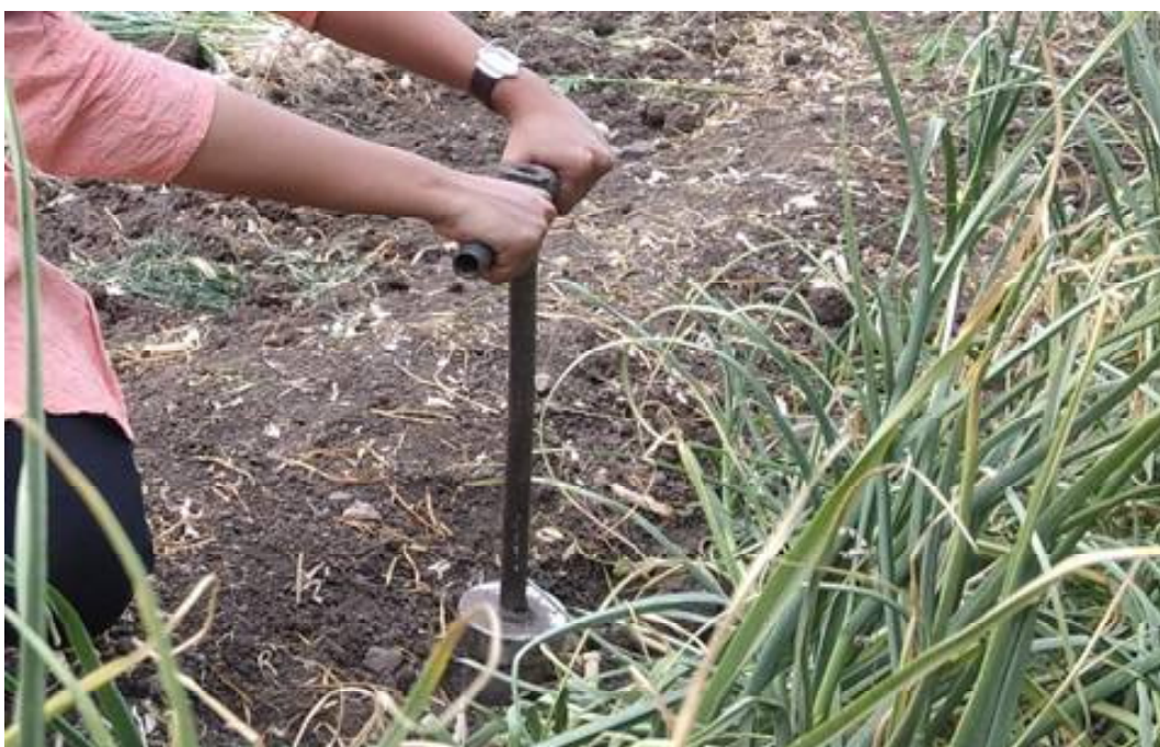
Fig. 6. Measurement of bulk density of soil
