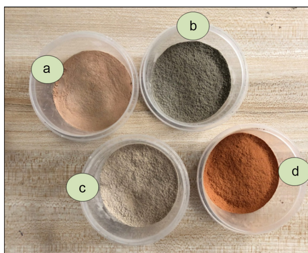
Figure 2. Binder materials used in this study: a) mixed waste powder; b) cement; c) waste concrete powder; d) waste brick powder.
