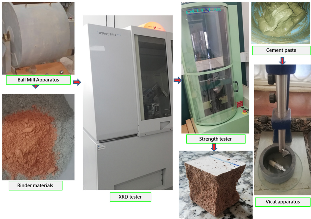
Figure 3. Procedure for the preparation of the WPs and equipment used in this paper at the National Center for Technical and Scientific Research (CNRST), Rabat, Morocco.
