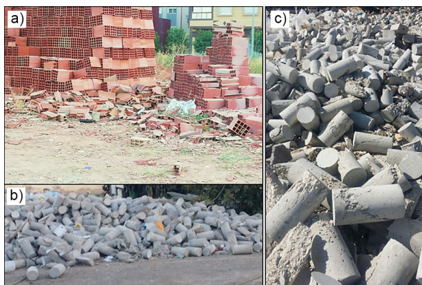
Figure 1. Types of construction and demolition waste (CDW) utilised in this research. Site of waste located in the city of Fez, Morocco: a) leftover brick waste; b) and c) landfill of concrete waste.
