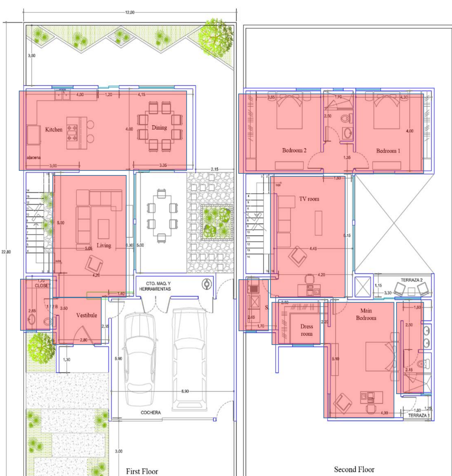
Fig. 2. Radiant floor heating surfaces
