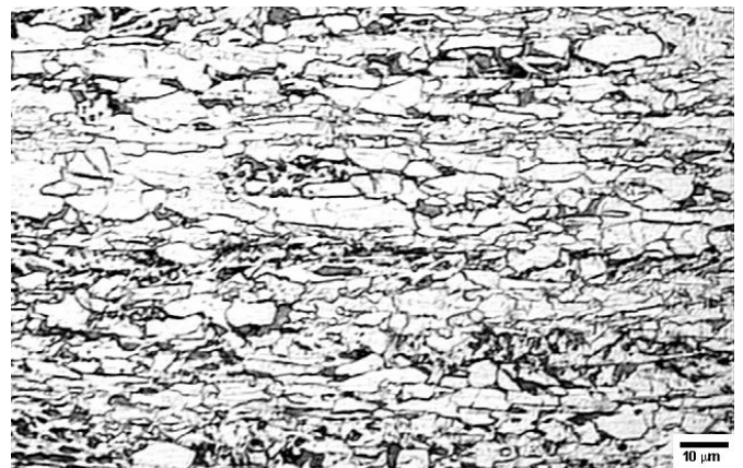
Figure 4- Original microstructure (tangent ends). Optical Microscopy. Magnification: 500X. Etch: 2% Nital.
