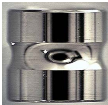
Figure 9: Inner Race of Unused Bearing
