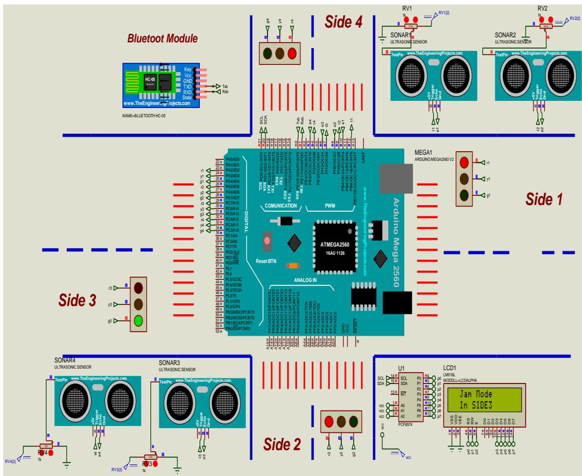
Fig.5 . The proposed system simulation using proteus
