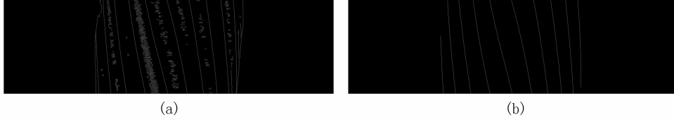
Fig. 4. (a). The stripe edges searched by the Canny edge detector. (b) The edge lines processed by the statistical and morphological algorithms.
