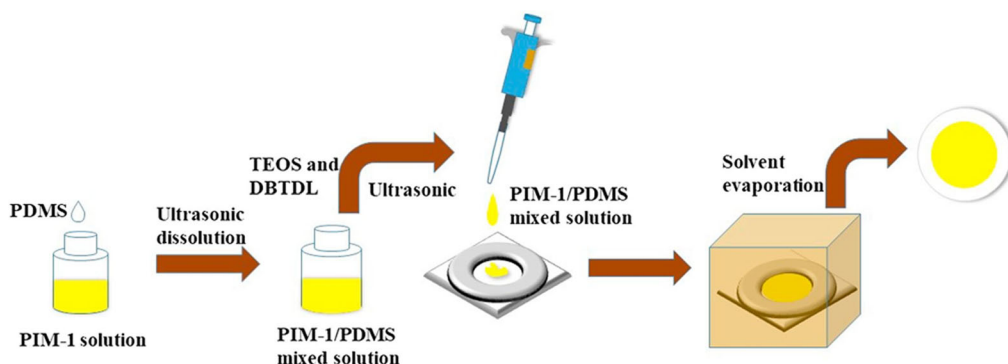
Figure 6. Preparation of PIM-1/PDMS membrane. 60
