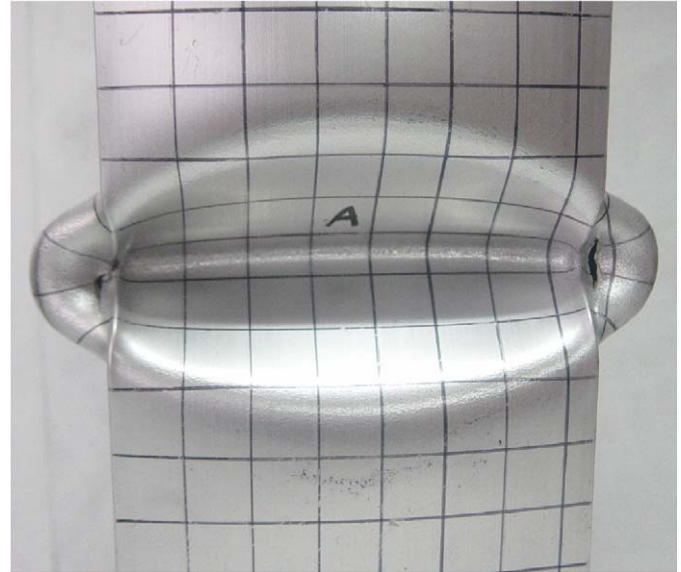
Fig. 3. Cracks taking place during crashing.
