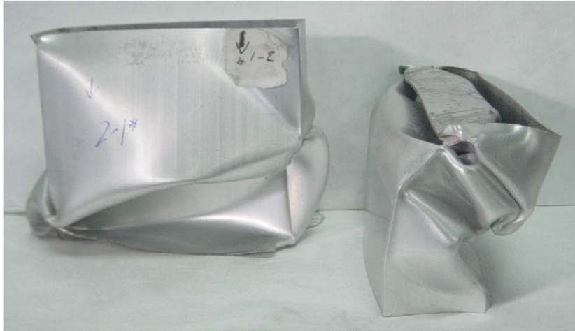
Fig. 5. Twist and band deformation modes dynamic crushing for thin-walled extrusion.
