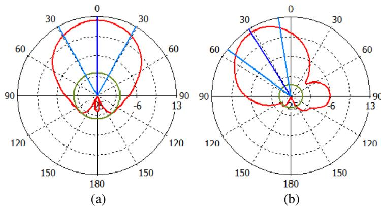
Figure 4: Bevel cut simulated gain patterns using CST without adding the reflector. (a) In the plane formed by the  $X$ -axis and the point of maximum radiation ( $\theta = \theta_m$ ,  $\phi = 90^\circ$ ). (b)  $\phi = 90^\circ$  plane.
