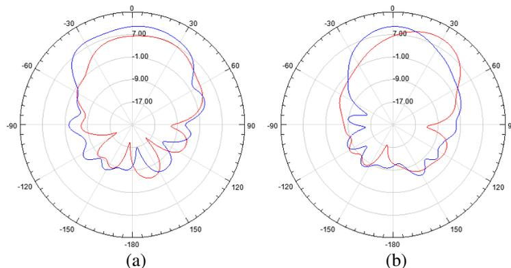
Figure 8: Step cut simulated gain patterns, with initial step-cut results shown in red and proposed design results in blue. (a) Red in the plane formed by the  $X$ -axis and the point of maximum radiation ( $\theta = \theta_m$ ,  $\phi = 90^\circ$ ), blue in  $\phi = 0^\circ$  plane. (b)  $\phi = 90^\circ$  plane.
