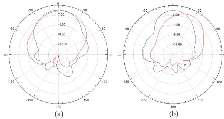
Figure 3: Simulated gain patterns computed using HFSS, with initial bevel-cut results shown in red and proposed design results in blue. (a) Red in the plane formed by the  $X$ -axis and the point of maximum radiation ( $\theta = \theta_m$ ,  $\phi = 90^\circ$ ), blue in  $\phi = 0^\circ$  plane. (b)  $\phi = 90^\circ$  plane.
