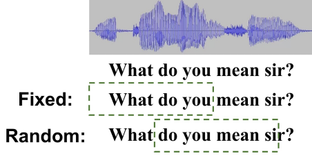
Figure 2: Two types of Boolean mask for acquiring linguistic information. The text bounded by the green dotted box corresponds to the mimicked speech clip.
