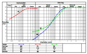
Figure 5. Grain size distribution curves of the studies soils samples
