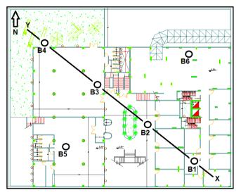
Figure 2. Layout of the studied project illustrated the studied boreholes (B1 to B6)
