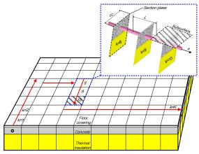
Figure 1 Illustration of space discretisation of a floor heating element with subsurfaces, section planes and pipe segments. The arrows indicate a conceivable pipe loop pattern. (Karlsson, 2006)
