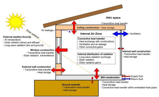
Figure 14 Schematic flow diagram for the general thermal problem with BIH. (Karlsson, 2006)
