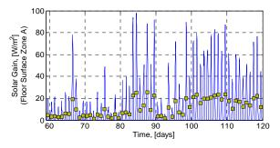
Figure 6 Solar radiation intensity; squares illustrate the diurnal average solar intensity that incident on the floor surface within Zone A.
