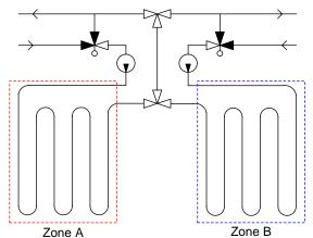
Figure 3 Principal system design for Case 1. Mixed return flows generates the desired heat transfer between A and B.
