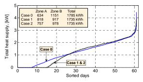
Figure 9 Total heat supply (Zone A and B together) to the floor heating pipe loops illustrated as a duration diagram. The inset illustrates the total amount of heat supplied in the all cases.
