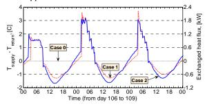
Figure 12 Total fluid temperature decline along the pipe loop within Zone A.
