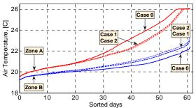
Figure 8 Duration diagram illustrating the indoor air temperatures during the 61 day period. The upper three lines are computed for Zone A, the other lines are for Zone B. Case 0 - solid, Case 1 dashed and Case 2 - dotted line.
