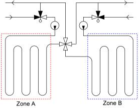
Figure 4 Principal system design for Case 2. The 4port valve interchange the system operation between two unique pipe loops or one single loop.
