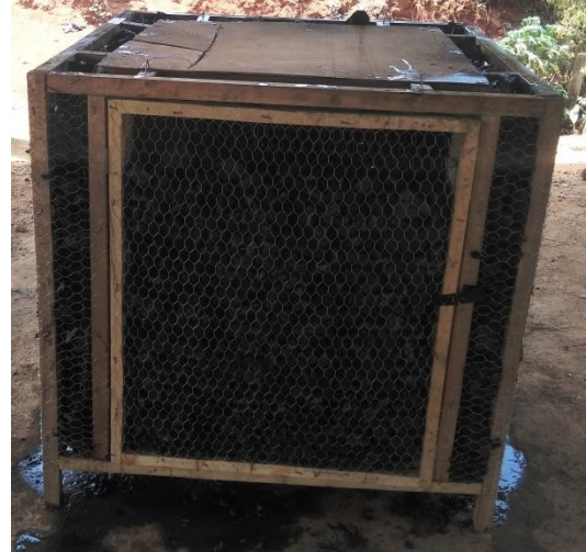
Fig. 5 Evaporative charcoal cooler put to use
