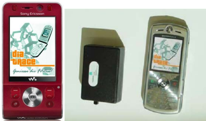
Figure 1. Modern electronic health technology consisting of a mobile motion sensor board (MoSeBo) (in the middle) or a wireless sensor for physical activity, integrated in a mobile phone with digital camera (DiaTrace) (left and right), developed by the Fraunhofer Institute for Graphical Data Management, IGD Rostock, Rostock, Germany.
