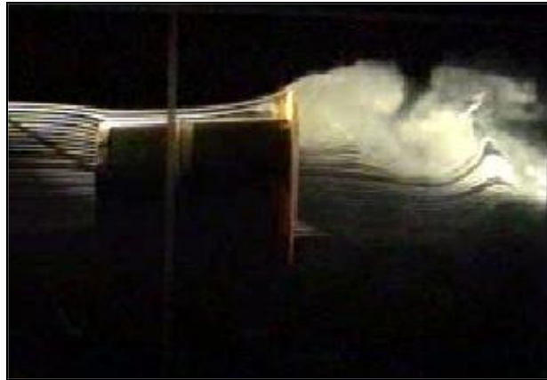
Figure 3: Flow simulation of flow within diffusers [9]
