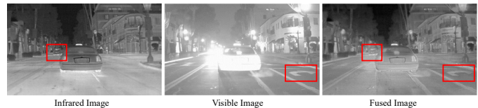
Fig. 1: An application example of infrared and visible image fusion in vehicle navigation.
