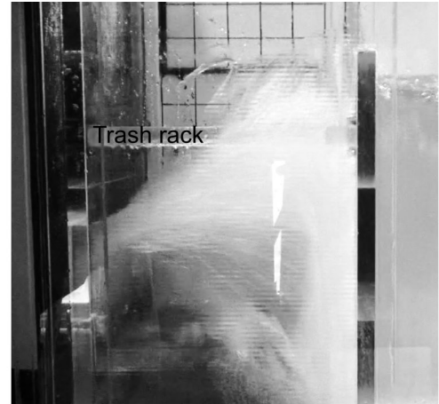
Figure 12: Opening of the intake gate with hydraulic pressure on one side. A jet hits the rack and the weir.
