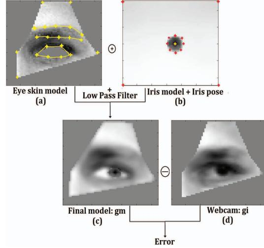
**Fig. 1.** Merging the eye skin model with the iris one to obtain the final model.
