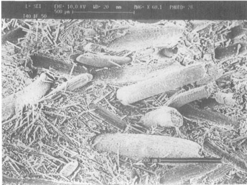
FIG. 11. Scanning electron micrograph for composites with 40% overall fiber content: 50% biofiber/50% glass fiber loading (magnification 60.1 \times ).
