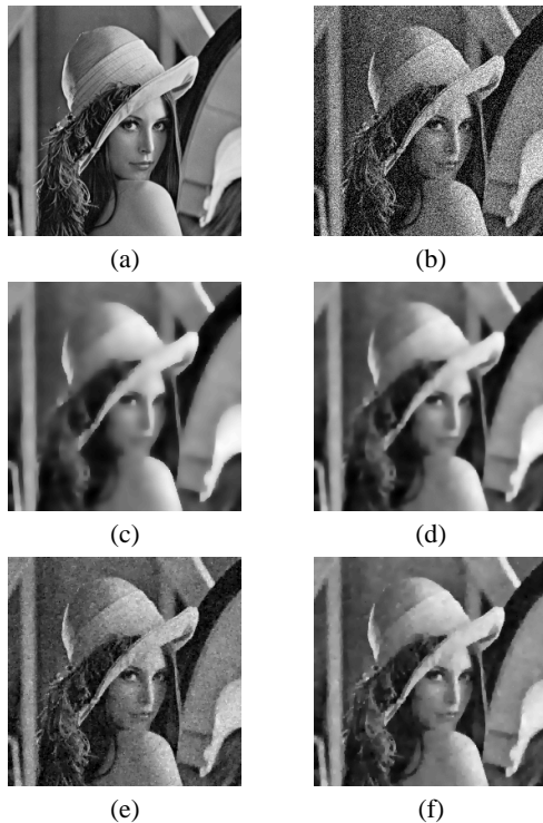
Fig. 2. Filtering results for Gaussian noise: (a) Original image, (b) Noisy image, (c) Huber flow, (d) Entropic flow, (e) Total Variation flow, and (f) Improved Entropic flow.
